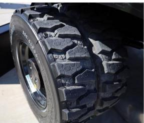
*Please note:* the original Power Grip 315/70R22.5 remains available to order as well. And due interference issues, both Caliber tyres cannot be ordered on ZX220W-7 with standard axles.
